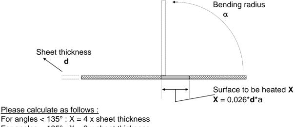
For angles >  $135^\circ$  : X = 2 x sheet thickness
