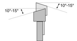
Type : **AKE16.300.2,9Z96** With inclination of teeth switching left, right, left, ...
