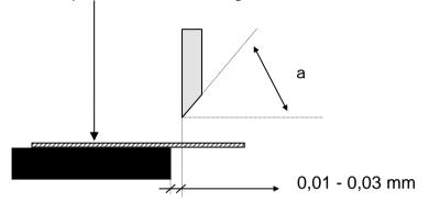
Always shear opposite to the extrusion direction.
