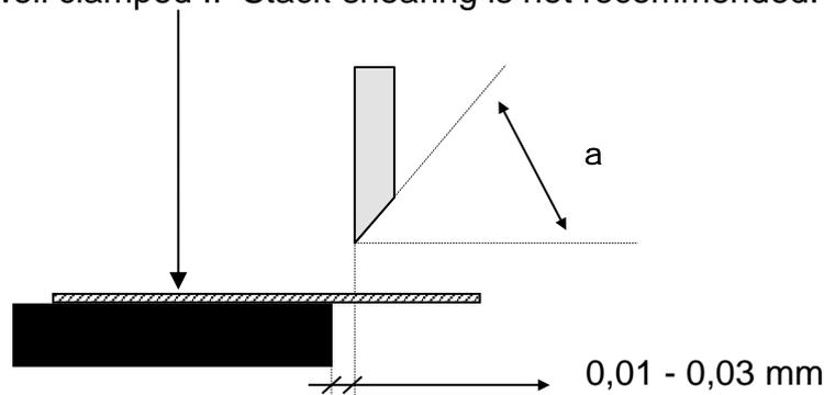
Always shear opposite to the extrusion direction.
