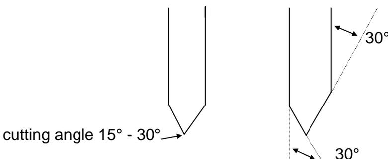
Diecutting presses have to be programmed to cut completely through the Veralite<sup>®</sup> sheet with a stroke that will prevent damaging the cutting rule. Proper testing is advised before starting production.
